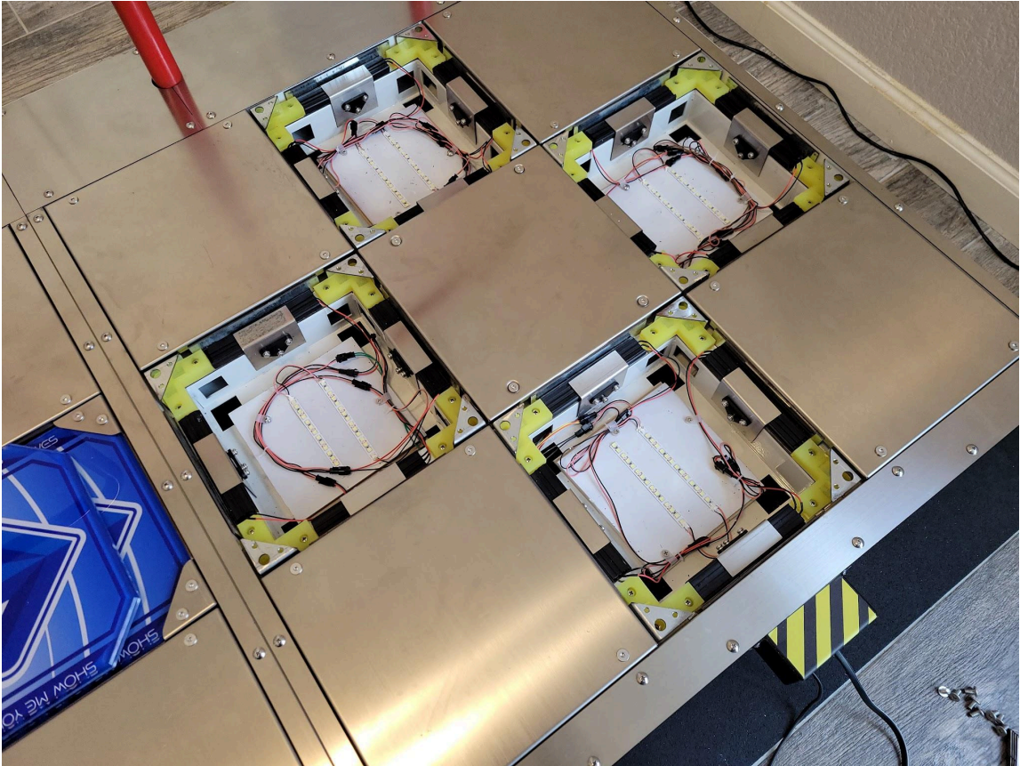
Open pad with all pre-installed foam removed
