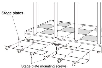
•Tighten the screws with the bottom face of stage plate being in contact with he floor.
